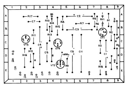
PRINTED CIRCUIT BOARD A.W.A. DRG. No. GO794W2 # T.C. WIRE # MOUNTED ON WIRING SIDE
